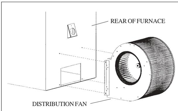
2. Attaching the distribution fan. First, remove the four (4) bolts from the rear of the unit. Secondly, slide the distribution fan up to the rear of the furnace, line up the (4) holes and reattach the bolts and tighten securely.
