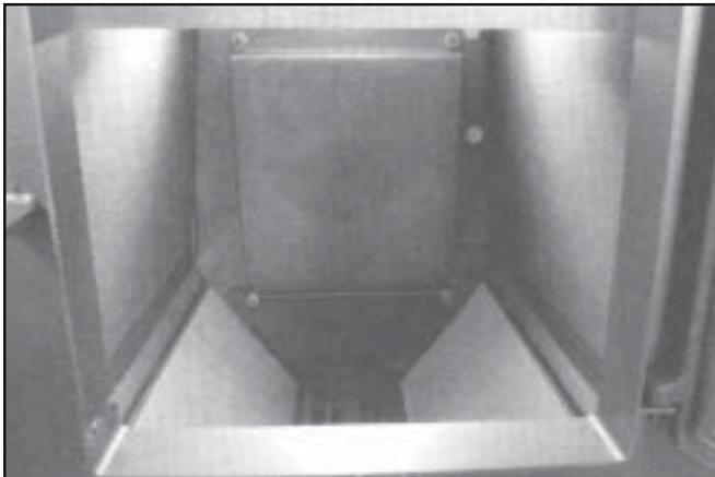
14. Now slip the rear heat plate in behind the rear baffle. Attach heat plate to the firebox by using two (2) 5/16 bolts, nuts & washers. First, line up the top holes and tighten bolts. Secondly, line up the holes in the rear baffle and the heat plate with the firebox and attach by using two (2) 5/16 bolts, nuts & washers. Tighten all four (4) bolts. NOTE: to reach rear bolts you may find it easier to put your arm through the flue outlet rather than to reach through the feed door.
