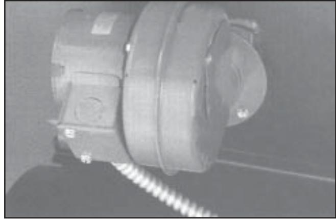
3. Attach the draft fan to the back of the weld on the throat (2" throat hole with 3 mounting holes). It's best to use the self tapping screws without the draft fan to establish threads then mount blower. The electrical box on the blower should be facing downward. Draft fan air intake cover should be set at a 20% opening, about 1/2" opening.
