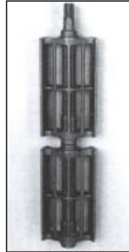
11. **Installing Grates:** Install grates together, slip shaker lug into hole and place grates into frame. Grate arch faces upward. Check out grate rotation by placing shaker handle on grate lug (3/4"). Grates should rotate freely.
