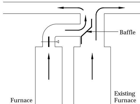
Your furnace is designed to be added on to existing duct work and operate either with or without another heat source such as a gas furnace. The following diagrams illustrate acceptable ways of ducting your furnace.
