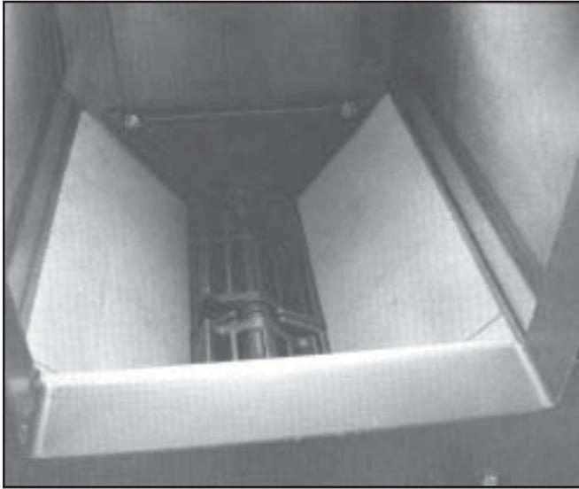
13. Installing front and rear cast baffles, heat plates.
