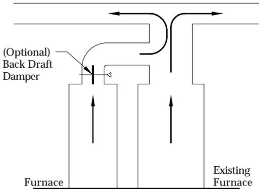
Chimney location is also critical. The furnace must be placed as close as possible to the chimney. You want the chimney connector (smoke pipe) to have a minimum of elbows, two (2) or less. Also, the chimney connector should not have to run more than six (6) feet to the chimney.
