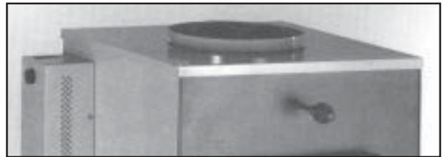
8. Install top shroud (if removed) by simply placing shroud on to the top of unit, push down, check each corner for snug fit.
