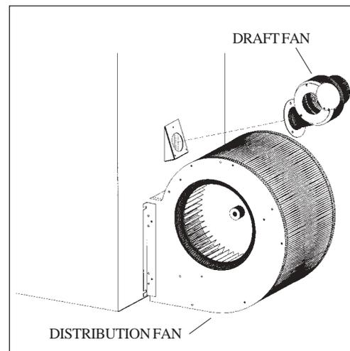
4. After mounting the two (2) fans proceed to the fan control center.
