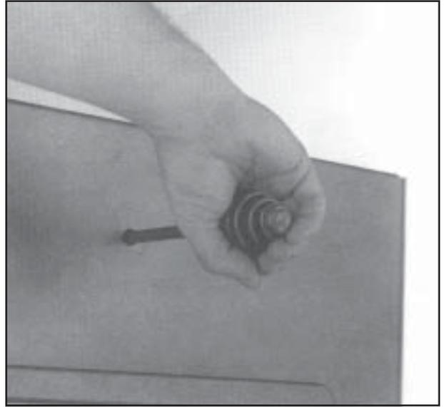
15. Installing smoke damper rod to sliding smoke damper. First, insert rod through hole above feed door and push forward.
