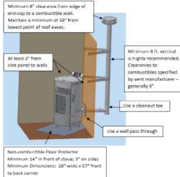
Locate terminations: a) not less than 3 feet above any forced air inlet located within 10 feet; b) not less than 4 feet below or horizontally from, or one foot above, any door, window or gravity air inlet; c) not less than two feet from an adjacent building and not less than 7 feet above a public walkway. Mobile home installations must use a spark arrester.
