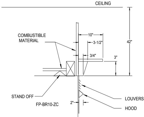
Bottom of 3/4" Base or Support must be Flush with top of Unit if mantel is 10" wide or less.
