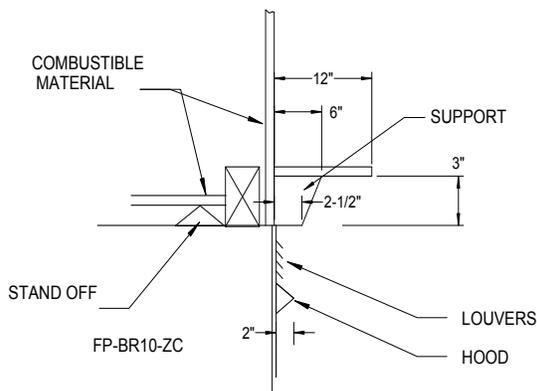
Bottom of 2-1/2" Base or Support must be Flush with top of Unit if mantel is 12" wide or less.
