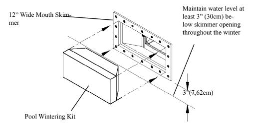
Insert the Pool Winterizing Kit (Part Number 1370138) into the skimmer until it fits flush with the skimmer flange. On some skimmers, it may be necessary to trim the foam to make a friction fit and/or use a wooden wedge to keep it in place during the winter.
