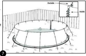
e. Cover the seam and bolt heads on the inside of the pool wall completely with three layers of 2" (50mm) duct tape.
