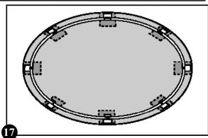
c. Remove the bottom rails and base plates and lay out the patio stones around the circle where the base plates were.
