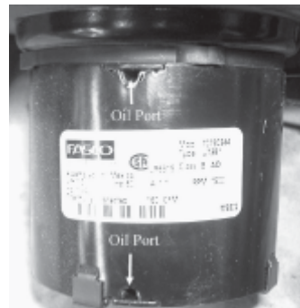
Figure 24. Oil ports on a circulation fan
