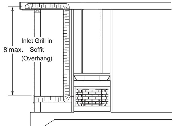
Figure 23 - Concrete Slab Installation (Optional Outside Air Runs)
