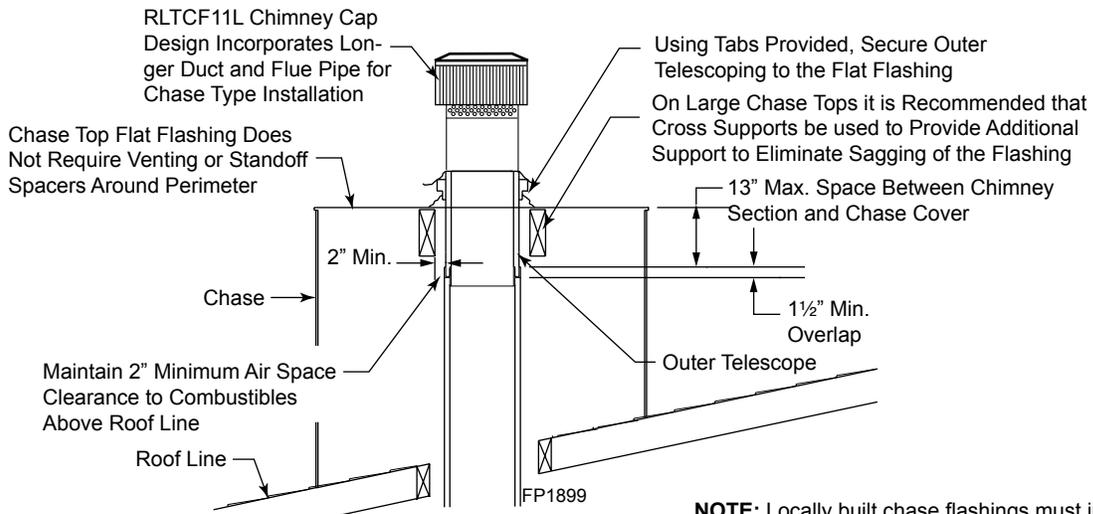
**NOTE:** Locally built chase flashings must incorporate a 1 3/4 min. to 1 3/4 max. x 2" high min. flanged hole for proper installation of the RLTCF11L chimney cap.
