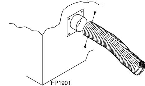
**Step 2:** Secure outside duct to starting collar with duct clamp or screws.
