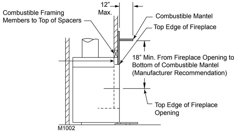
**NOTE:** If Model WSB60 glass doors are to be used, noncombustible trim attached to the face of the fireplace must not extend over the screen cover at the top of the firebox opening. The screen cover will have to be removed before model WSB60 glass doors can be installed. Noncombustible trim must not extend over each side of the fireplace into the firebox opening to avoid interference with installation of the model WSB60 glass doors.
