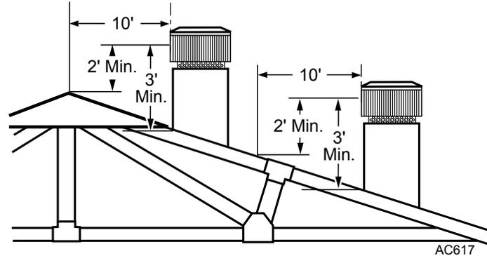
**NOTE:** Flue outlet should be two feet above all portions of the building within ten feet as shown in Figure 17. The chimney must not extend more than 90 inches above the roof without additional support.
