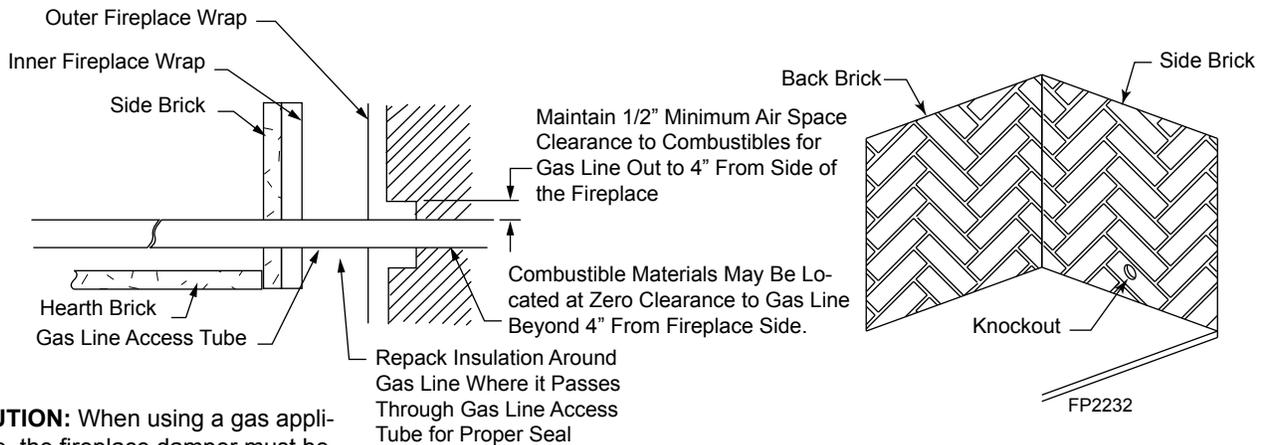
**CAUTION:** When using a gas appliance, the fireplace damper must be set in fully open position.
