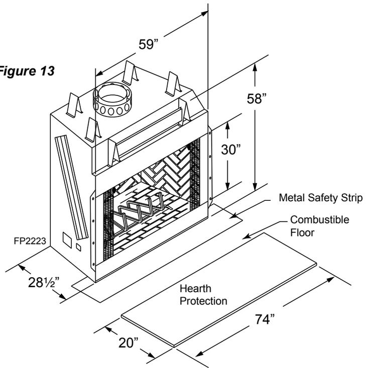
**WARNING:** The hearth extension and the metal safety strip should be installed only in a horizontal relationship to the fireplace.
