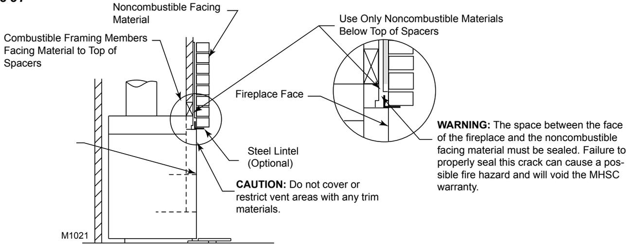
**CAUTION:** Do not allow any trim materials to extend closer than 3/8 inch to the vertical edges of the firebox opening if glass doors are to be installed.
