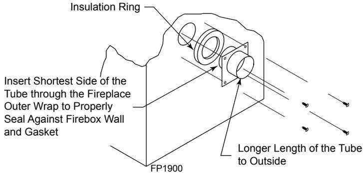
**Step 1:** Secure outside air starting collar to left side of fireplace with four (4) sheet metal screws provided.
