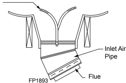
**NOTE:** Although both halves of the elbow set may have tie straps, only the top half must be secured. The bottom elbow half is not required to be secured for added stabilization of pipe.
