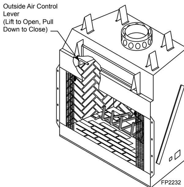
**MODEL AK-4 COMBUSTION AIR ASSEMBLY**
