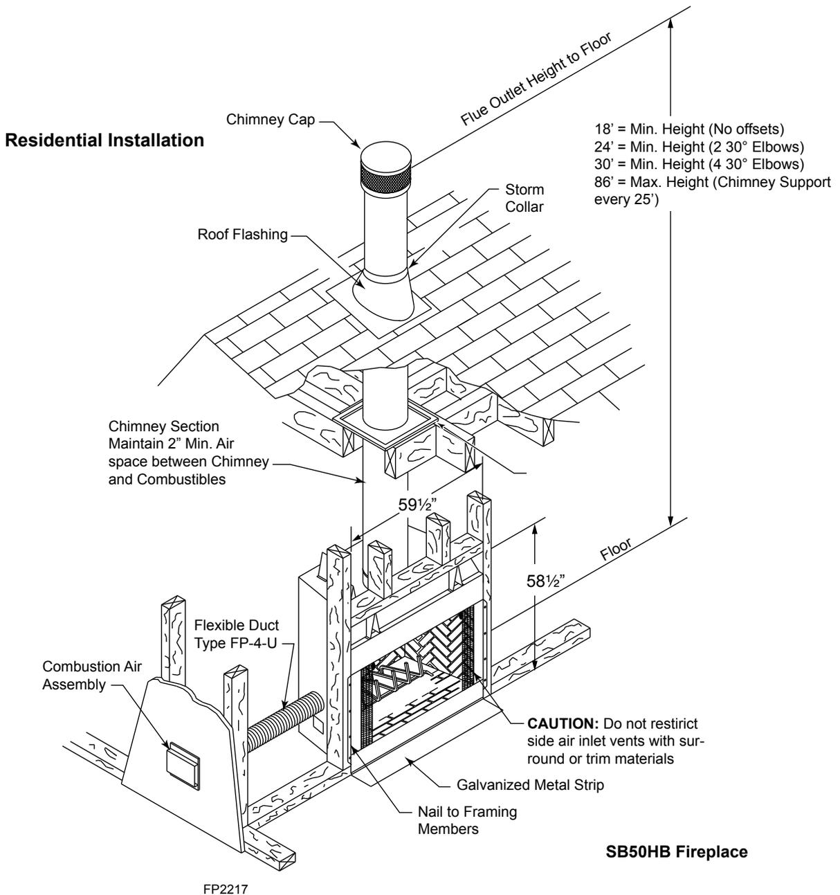
**NOTE:** If Model WSB60 glass doors are to be used, noncombustible trim attached to the face of the fireplace must not extend over the screen cover at the top of the firebox opening. The screen cover will have to be removed before Model WSB60 glass doors can be installed. Non-combustible trim must not extend over each side of the fireplace into the firebox opening to avoid interference with installation of the Model WSB60 glass doors.
