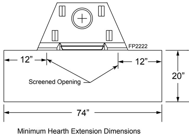
**NOTE:** A hearth extension placed on a combustible floor must be constructed with rigid insulation which has a minimum "R" value of 1.16 or a "K" value of 0.43. The insulation must be covered with a noncombustible covering such as a tile, stone, marble, or a piece of 0.018 minimum sheet metal which is needed to protect the insulation. Follow instructions provided with the for all other specifications and directions for proper installation of the fireplace and hearth extension.
